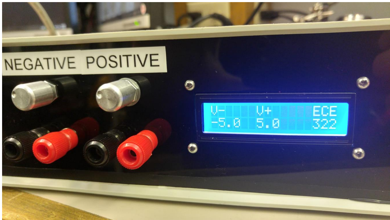
Figure 16: Picture of the Display measuring the voltage on the Power Supply
